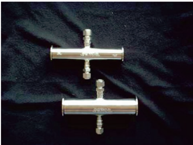
Fig.3: Flow cells with different diameters for absorption spectroscopy
