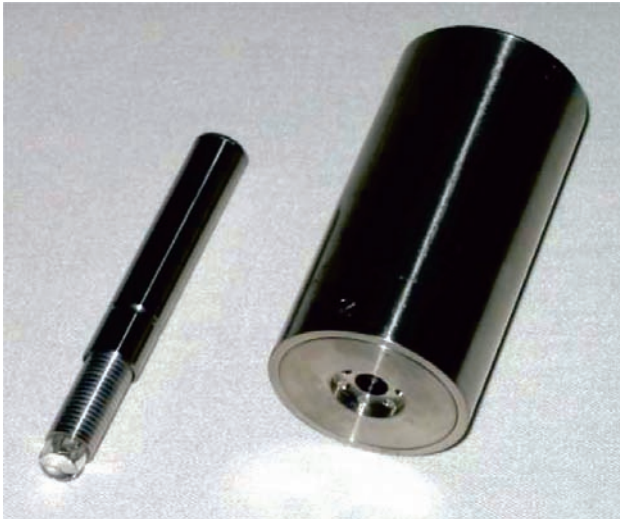
Fig.2: Measurement head with light source for reflection spectroscopy
