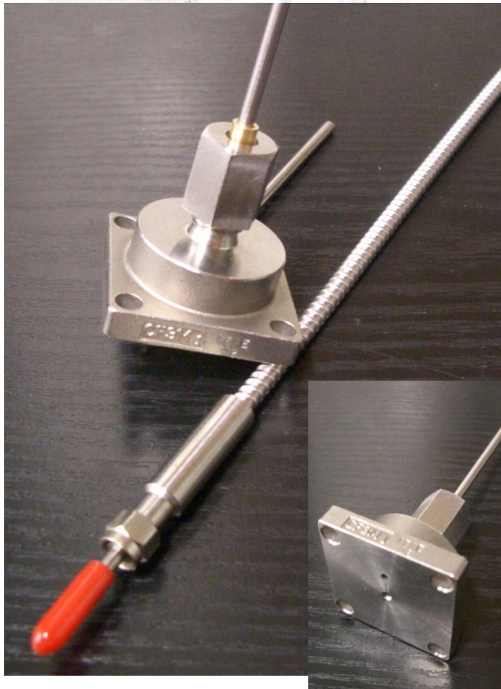
Diamond ATR-IR-Fiber Probe of 2.7mm diameter in NeSSI
