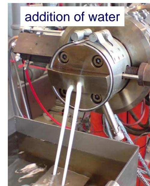
Determination of particle size of  $\text{TiO}_2$  with different water content during extrusion
