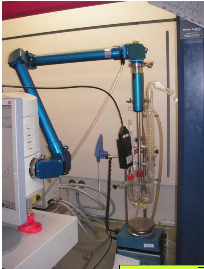
**ATR-IR spectrometer:** ReactIR 4000 (Mettler Toledo)
