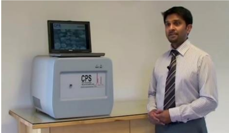
Picture: DC24000 ultra high-resolution particle size analyser 'in action'
