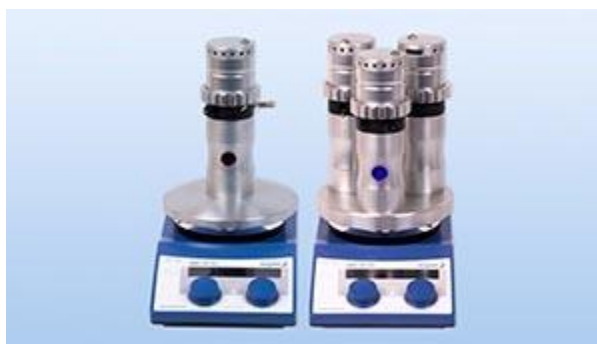
Image caption; Single position and 3-position LightSyn Lighthouse photoreactor
