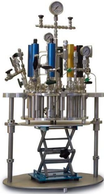
Caption: Multicell PLUS and close-up of easy-to-use support frame / lifting platform option
