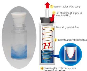
*Solvent evaporation specialists - BioChromato Inc. has published an informative web page that describes how Vacuum Vortex Concentration (VVC) methodology enables users of its Smart Series of Evaporators remove even higher boiling solvents including water, DMSO and DMF quickly and safely.*
