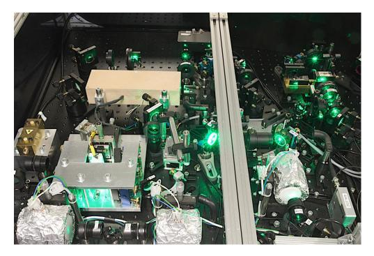
Macroscopic trial set-up for complex laser systems in an optical atomic clock. © Ulrich Rosowski, Heinrich Heine University of Düsseldorf Print quality: <a href="https://www.izm.fraunhofer.de/pics">www.izm.fraunhofer.de/pics</a>
