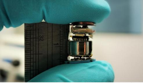
The core of the spectroscopy capsule contains the system-in-package, a flexible circuit board, and a ceramic pcb © Fraunhofer IZM, image in print quality: www.izm.fraunhofer.de/pics
