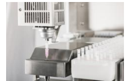
Gripper injects SMART column in ThermELUTE module.
